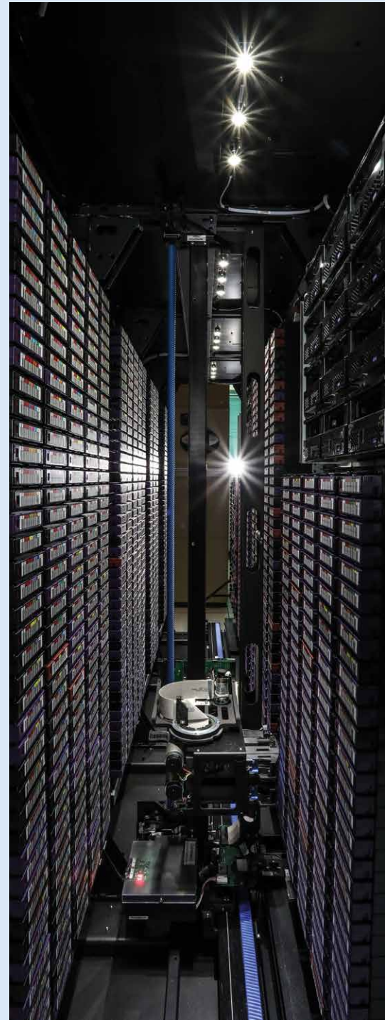
Photo: The IBM 3584 tape robot at OSC's data center provides more than 23.5 petabytes of highly reliable and secure backup storage.
